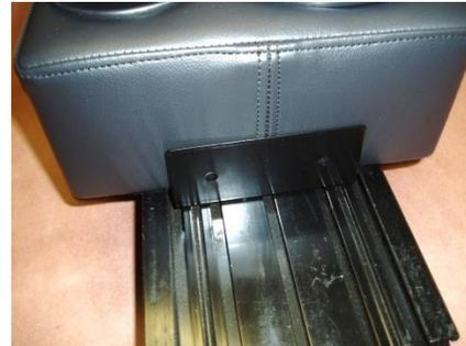
3. Slide the right angle brackets snug up to the console body.
